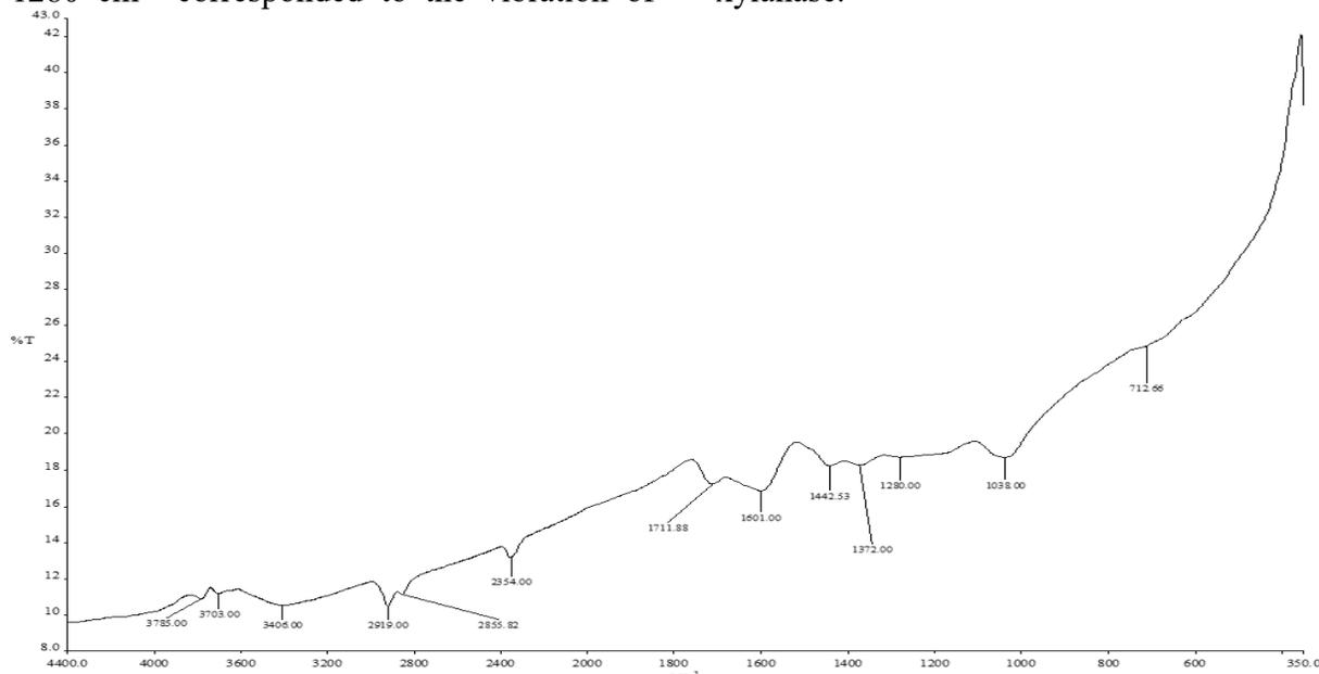
**Figure 3:** FTIR spectra of biosynthesized of biosynthesized AF5L-AgNPs.
