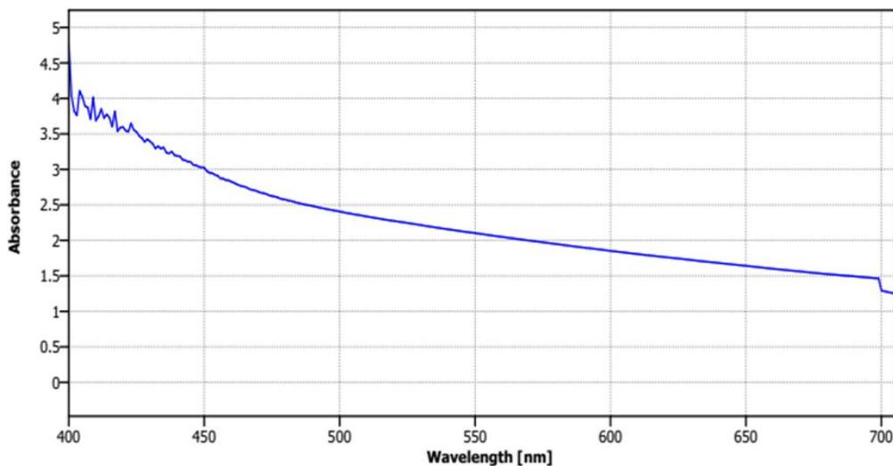
**Figure 2:** UV-Vis absorption spectra of biosynthesized AF5L-AgNps
