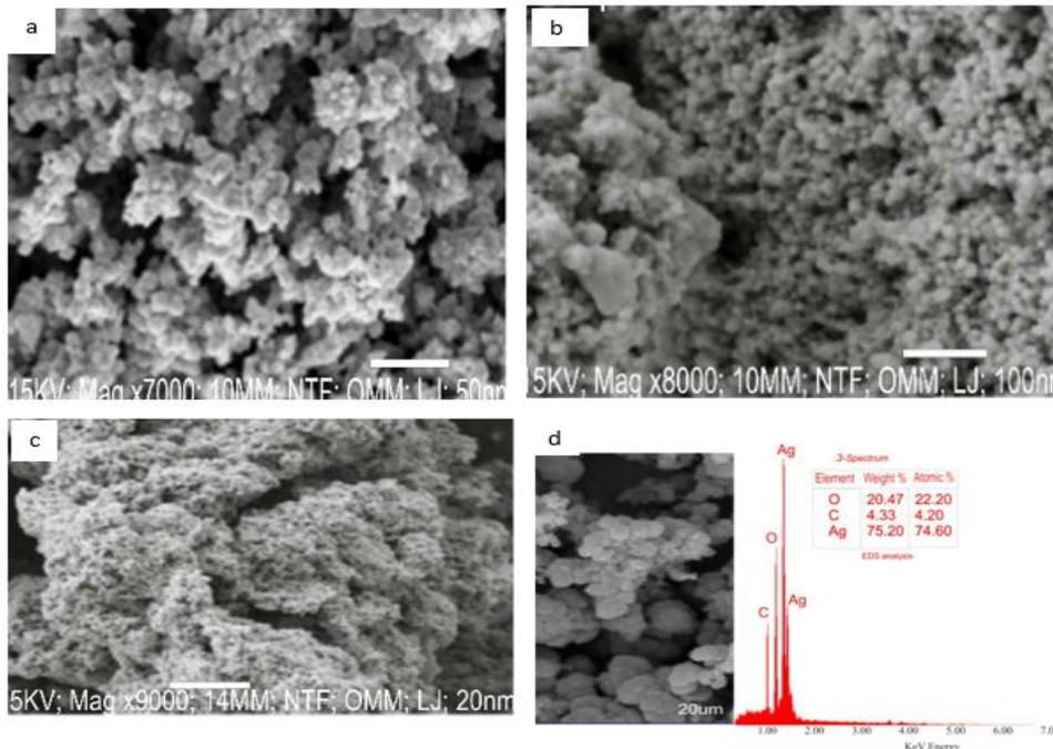
**Figure 4:** SEM analysis of biosynthesized AF5L-AgNPs 50 nm with Mag x 7000 (a), 100 nm with Mag x 8000 (b), 20 nm with Mag x 9000 (c), EDS spectrum of biosynthesized AF5L-AgNPs (d)
