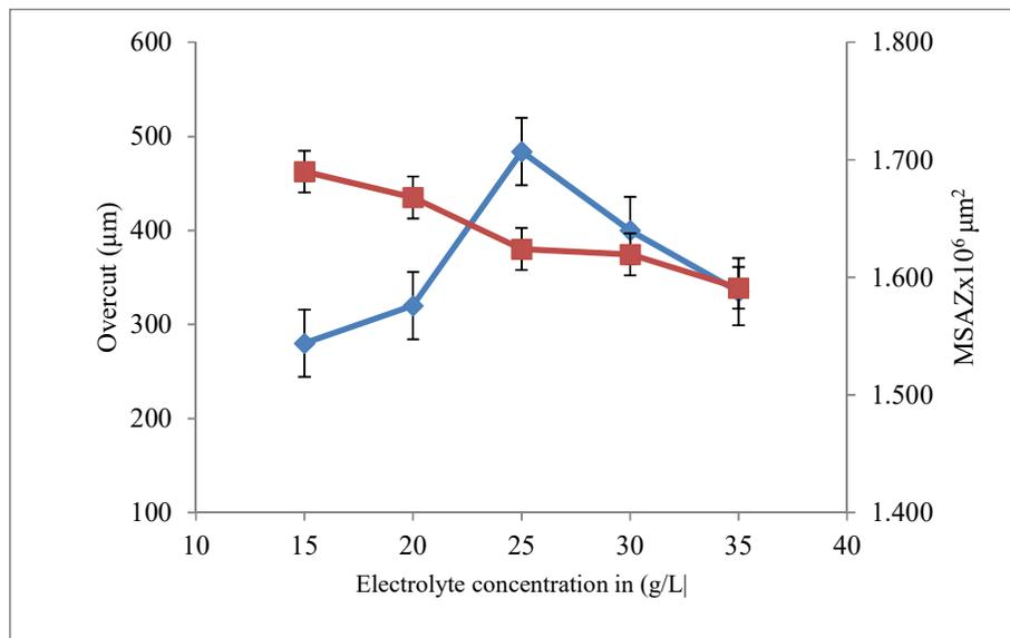
Figure 6. Electrolyte Concentration vs overcut, MSAZ.
