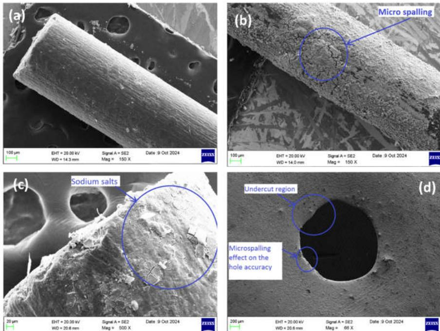
Figure 7. Electrode condition (a) before machining, (b) after machining (10 V, 35 g/L and 50% duty cycle), (c) electrode with salt deposition, and d) hole with micro-spalling effect.
