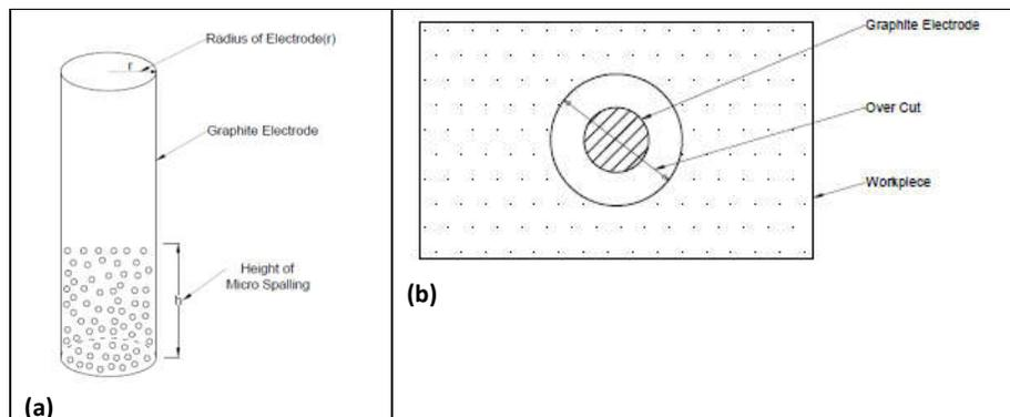
Figure 4. (a) Sketch of graphite electrode with micro-spalling and (b) overcut in the work piece.
