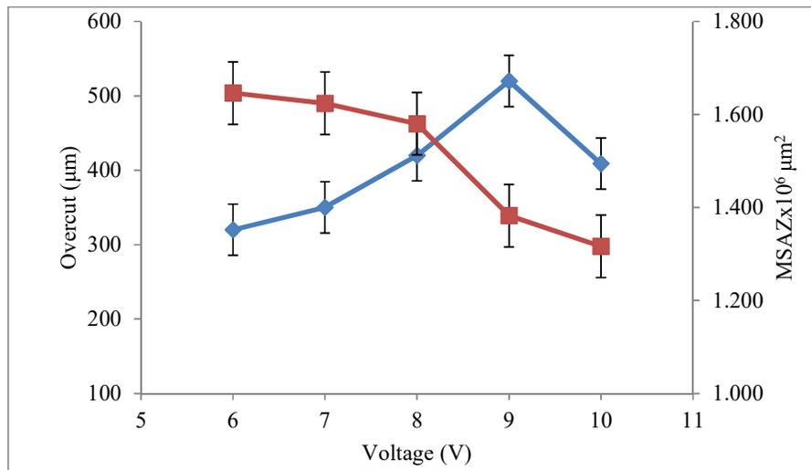
Figure 5. Voltage vs overcut, MSAZ.
