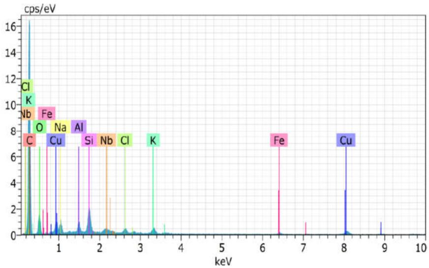
Figure 2. EDAX of Graphite electrode.
