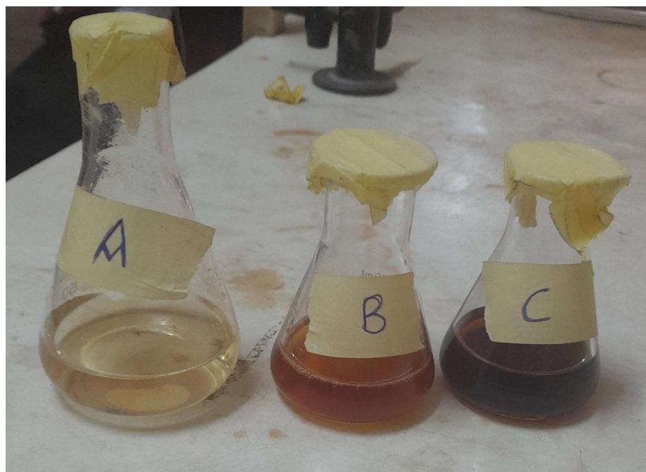
Figure 2. (a) CFE of the yeast isolate after agitation of broth for 48 hours, (b) CFE with 3 mM \text{AgNO}_3 at 12 hours and (c) Synthesized silver nanoparticles after 72 hours.
