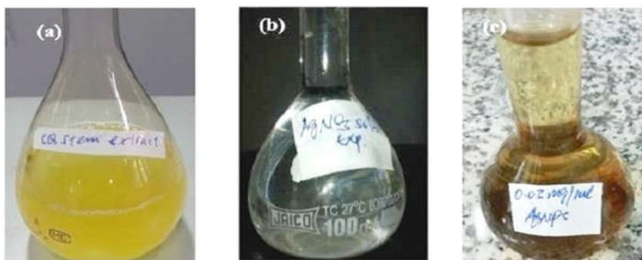
Figure 4. The color changes of the samples (a) yellow color of the aq. extract of the Cissus quadrangularis stem aq. Extract, (b) \text{AgNO}_3 solution and (c) dark brown color of AgNP formation.
