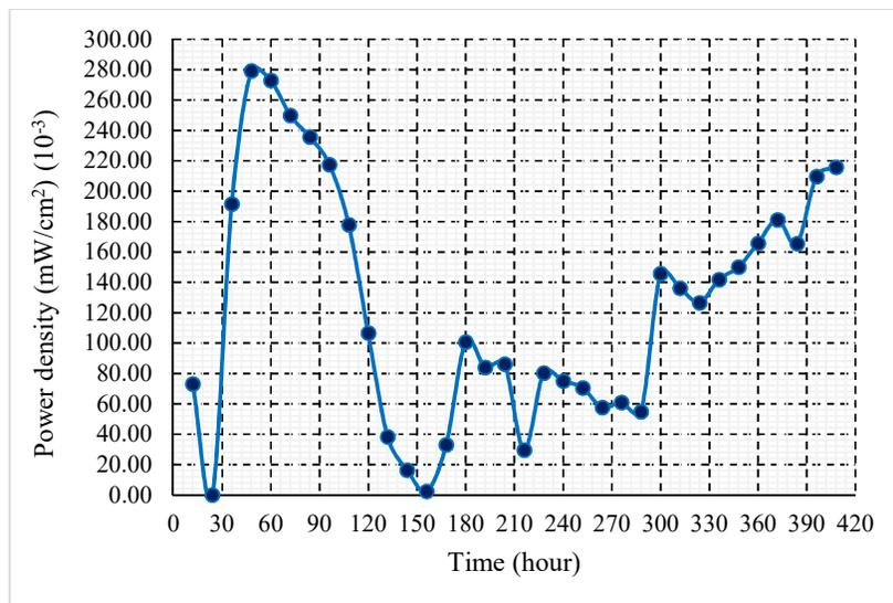
Figure 7. Maximum power densities of the system (from minimum internal resistance).
