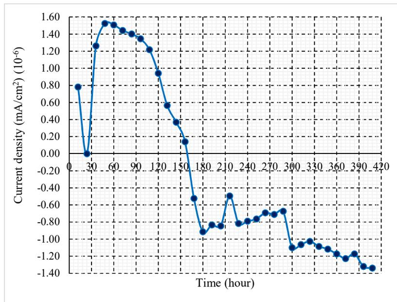
Figure 6. Minimum current density of the system (from minimum internal resistance).
