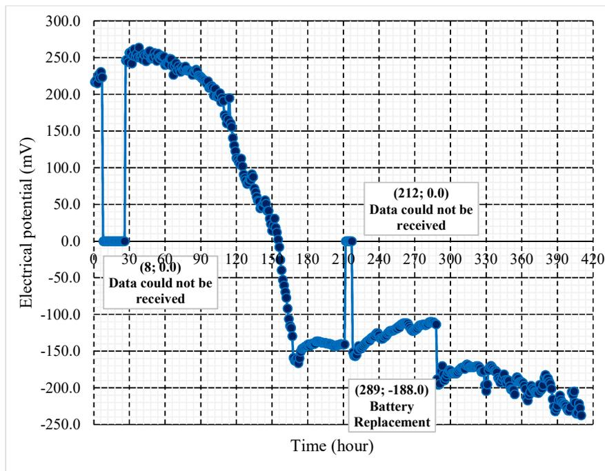
Figure 4. Electrical potential measurements of the system.
