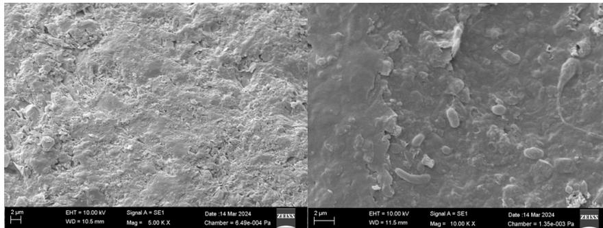
Figure 2. SEM analysis of the sediment without (left one) and with (right one) native microorganisms.
