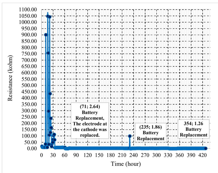
Figure 3. System resistance measurements.
