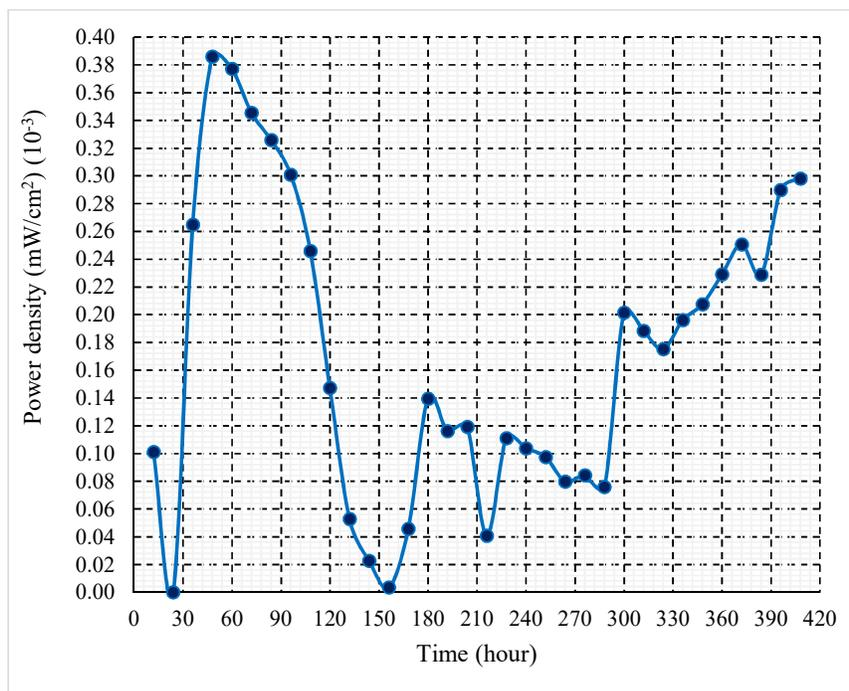
Figure 8. Minimum power density of the system (from minimum internal resistance).
