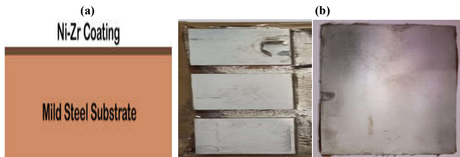
Figure 2. (a) Coating architecture and (b) as-coated specimens.
