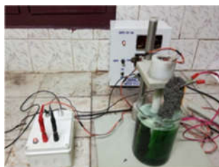
Figure 1. Electroplating setup for co-deposition.
