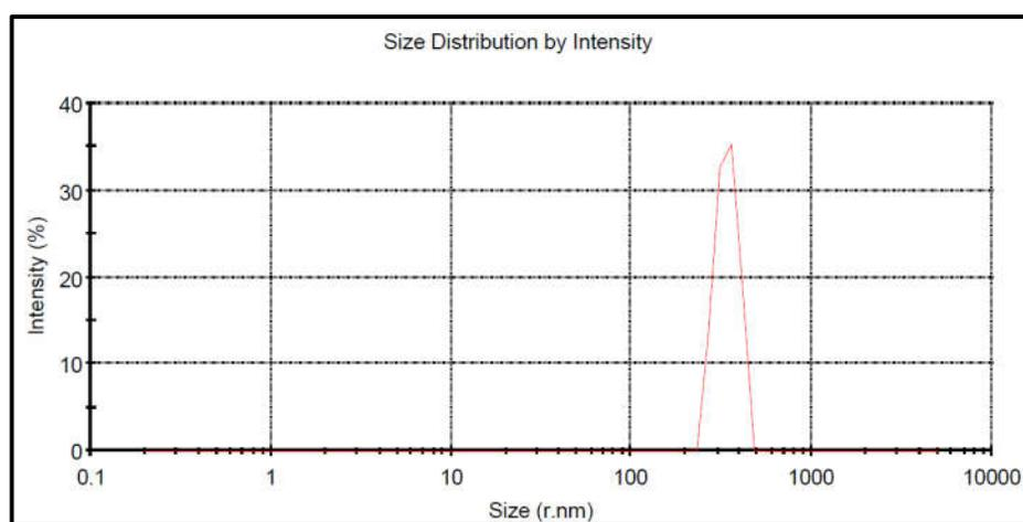
Figure 3. Dynamic light scattering (DLS) spectrum showing the  $\gamma$ -Al<sub>2</sub>O<sub>3</sub> NPs size distribution.
