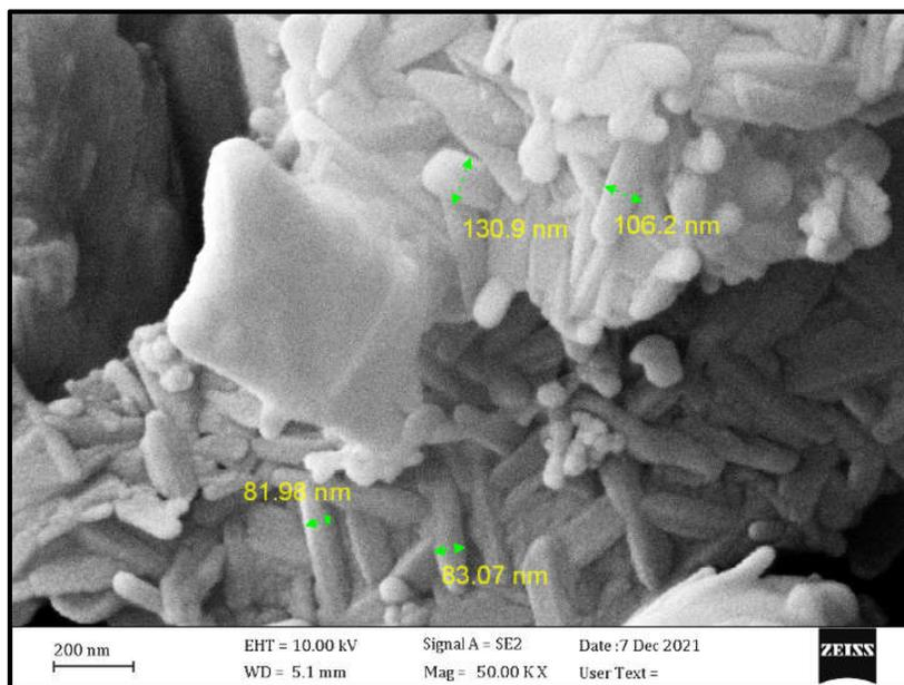
Figure 2. FE-SEM image of  $\gamma$ -Al<sub>2</sub>O<sub>3</sub> NPs.
