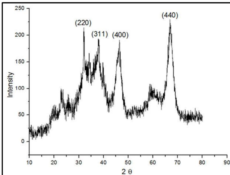
Figure 1. XRD diffraction pattern of  $\gamma$ -Al<sub>2</sub>O<sub>3</sub> NPs.
