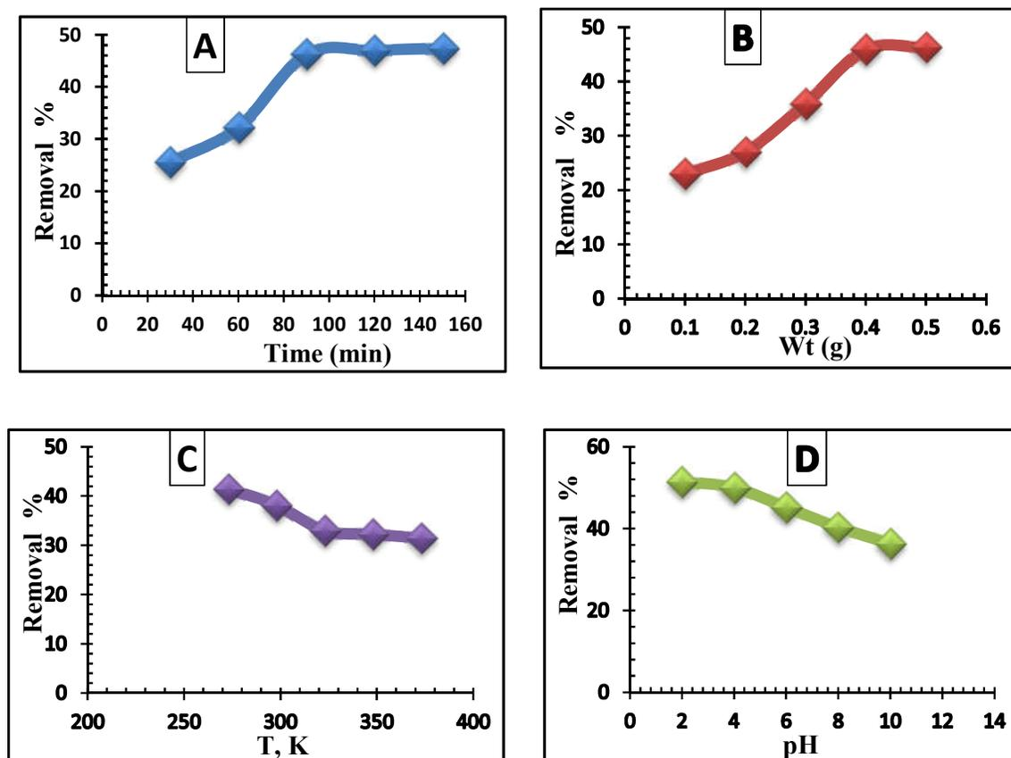
Figure 5. Shows the removal % of sulfur compounds versus (A) contact time, (B) weight of  $\gamma$ - $\text{Al}_2\text{O}_3$ , (C) temperature and (D) pH.
