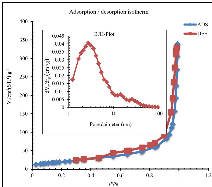
Figure 4.  $\gamma$ - $\text{Al}_2\text{O}_3$  nanoparticles  $\text{N}_2$  adsorption-desorption isotherm (Inset: Pore size distribution curves).
