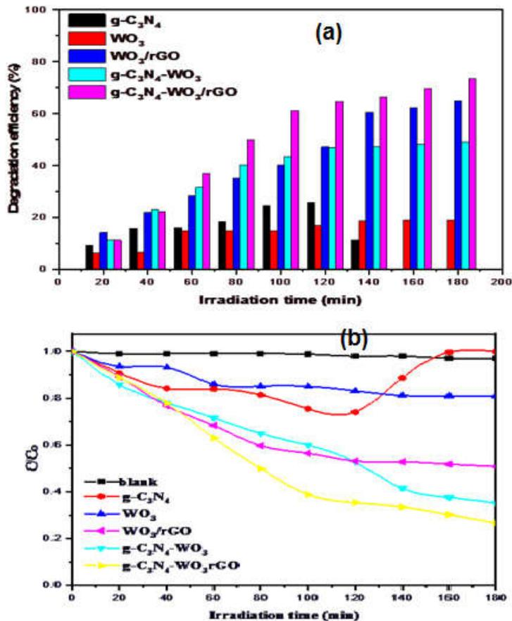
Figure 5. Degradation rate (a) and visible light driven photogradation of methylene blue (b) using g-C<sub>3</sub>N<sub>4</sub>, WO<sub>3</sub>, WO<sub>3</sub>/rGO, g-C<sub>3</sub>N<sub>4</sub>-WO<sub>3</sub> and g-C<sub>3</sub>N<sub>4</sub>-WO<sub>3</sub>/rGO.
