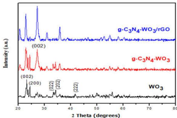
Figure 2. Powder XRD of pure, binary and ternary composite of tungsten oxide.
