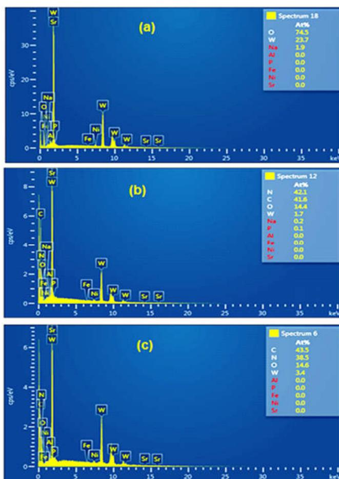
Figure 4. EDX spectra (a) Pure  $\text{WO}_3$ , (b)  $\text{g-C}_3\text{N}_4\text{-WO}_3$  and (c)  $\text{g-C}_3\text{N}_4\text{-WO}_3/\text{rGO}$ .
