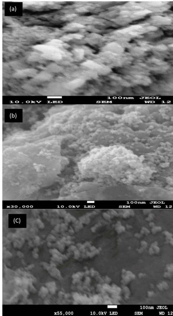
Figure 3. Scanning electron microscopy images (a) Pure WO<sub>3</sub>, (b) g-C<sub>3</sub>N<sub>4</sub>-WO<sub>3</sub> and (c) g-C<sub>3</sub>N<sub>4</sub>-WO<sub>3</sub>/rGO.
