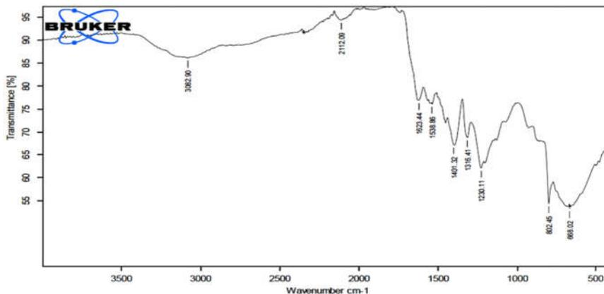
Figure 1. FT-IR Spectrum of  $g\text{-C}_3\text{N}_4\text{-WO}_3/\text{rGO}$  ternary composite.
