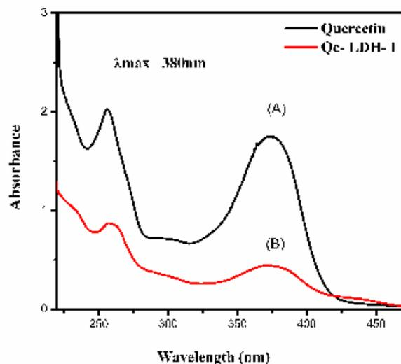
Figure 7. UV-visible spectra of QC & QC-LDH-I.
