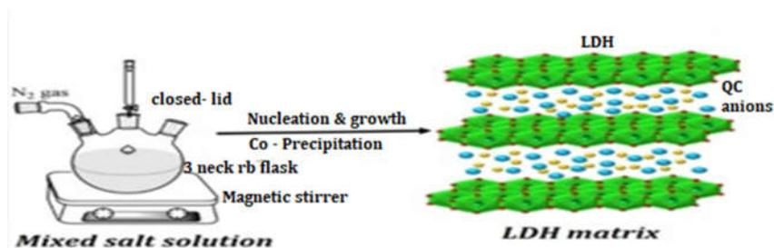
Figure 2. Schematic representation of co-precipitation method.
