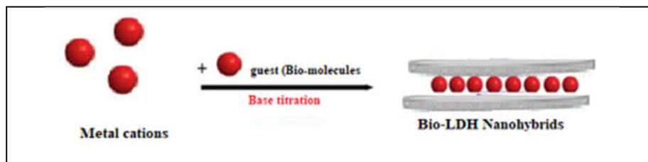
Figure 4. Intercalation routes to layered nanohybrids co-precipitation.
