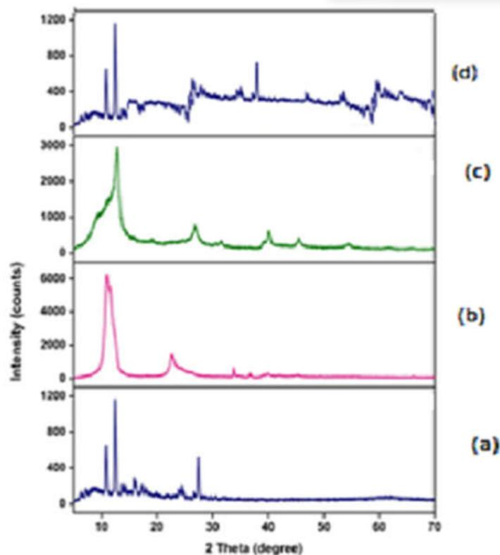
Figure 5. (a) XRD patterns of quercetin, (b) XRD patterns of LDH, (c) XRD patterns of QC-LDH by ion-exchange method and (d) XRD patterns of QC-LDH by co-precipitation method.
