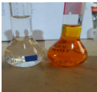
Figure 4. From traditional laboratory bench to lab-on-a-paper device. Reaction of PHP (0 and 12.5 mg L -1 ) with DSDM in alkaline conditions to produce an orange azo-dye done on paper-based microfluidic analytical devices ( \mu PADs).
