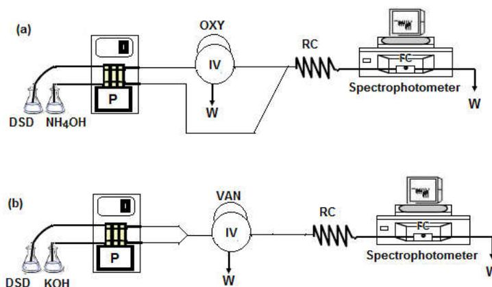
Figure 1. A diagram of the CFI manifolds for (a) OXY and (b) VAN; IV, injection valve; P, peristaltic pump; FC, flow cell; RC, reaction coil; W, waste.
