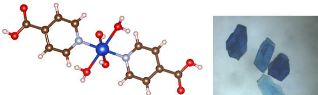
Fig. 1(a): Connectivity and coordination environment of Cu in [Cu(INA) 2 (OH) 2 (H 2 O) 2 ]. (Cu = Blue, O = Red, N = Grey, C = Brown, H = Pink). (b): Microscope of [Cu(INA) 2 (OH) 2 (H 2 O) 2 ]
