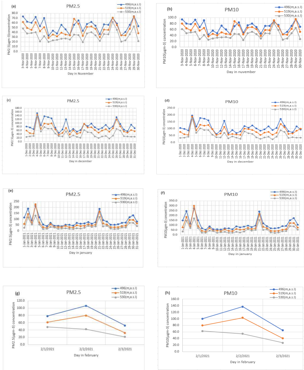
Figure 2a-h: Daily variations of PM 2.5 and PM 10 concentration at 496, 519, and 530 (m.a.s.l) heights over all days of measurement during observation period (from 3 rd November 2020 to 3 rd February 2021)
