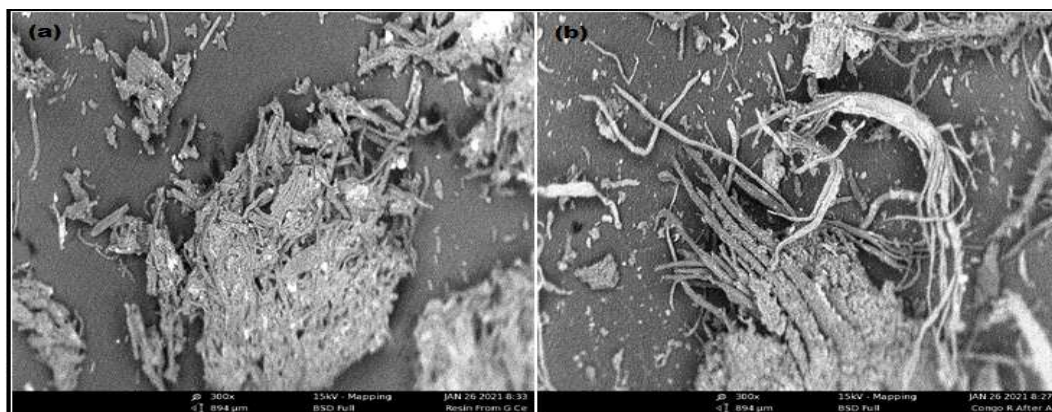
Fig. 4 SEM image of (a) poly(amidoxime) ligand, (b) poly(amidoxime) ligand after Congo red dye adsorption
