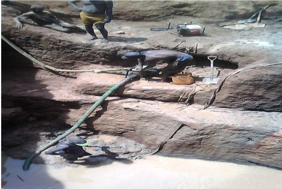
Plate 1: Miners draining water from a mine pit Source: Field Survey, 2019
