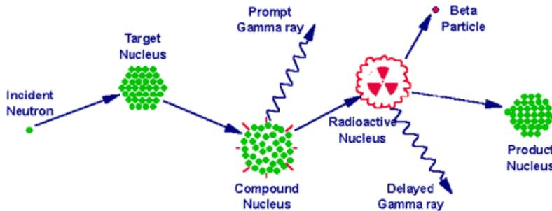
Figure 1: Neutron capture by a target nucleus followed by the emission of gamma rays [21]
