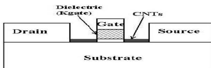
Figure 1: Carbon nanotube FET
