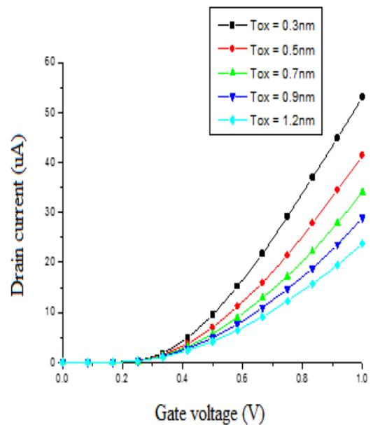
Figure 4. Graph of drain current against gate voltage for different oxide thickness in silicon nanowire MOSFET
