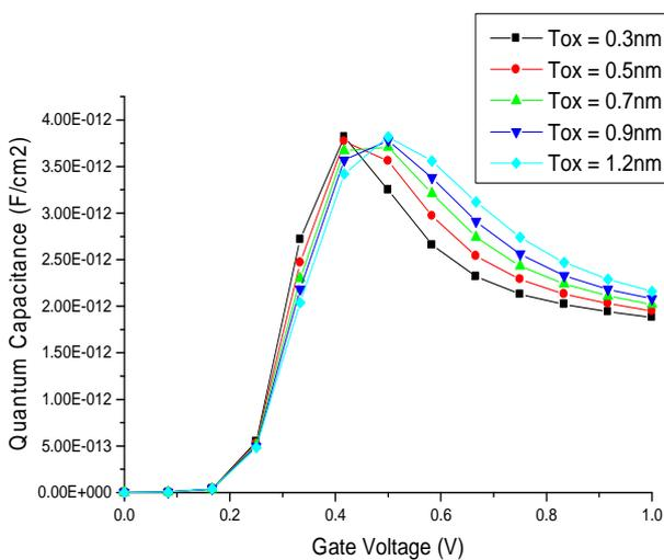
Figure 5: A graph of quantum capacitance against gate voltage for different oxide thickness in carbon nanotube MOSFET
