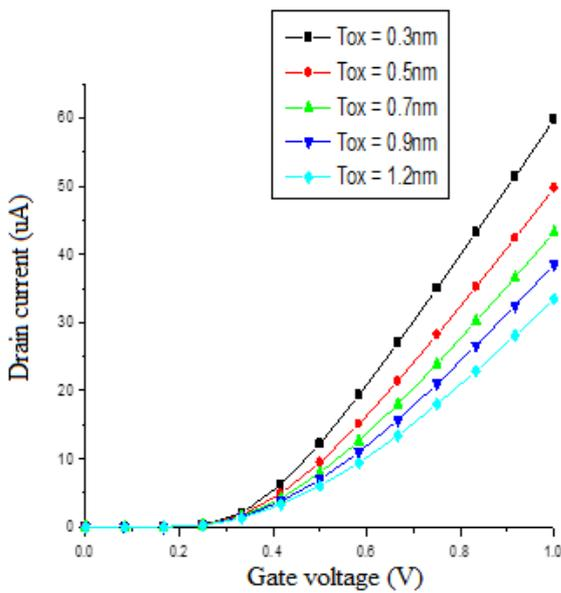
Figure 3. Graph of drain current against gate voltage for different oxide thickness in carbon nanotube MOSFET
