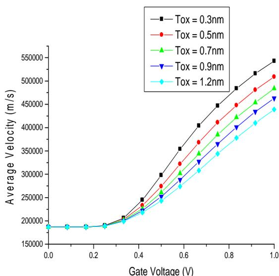
Figure 7: A graph of average velocity against gate voltage for different oxide thickness in carbon nanotube MOSFET
