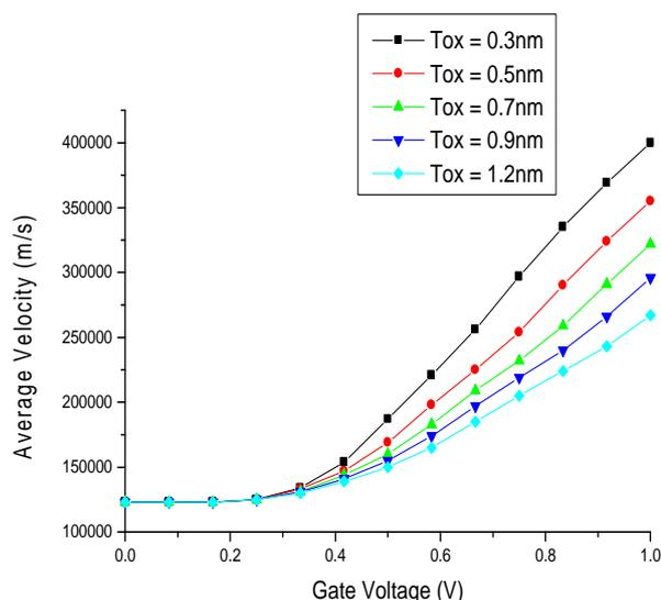
Figure 8: A graph of average velocity against gate voltage for different oxide thickness in silicon nanowire MOSFET
