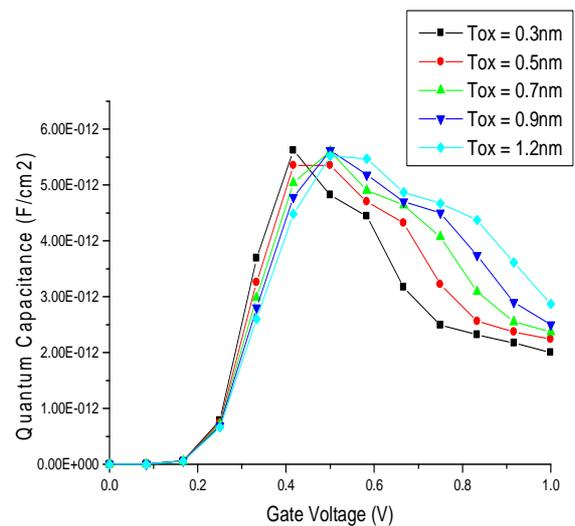
Figure 6: A graph of quantum capacitance against gate voltage for different oxide thickness in silicon nanowire MOSFET
