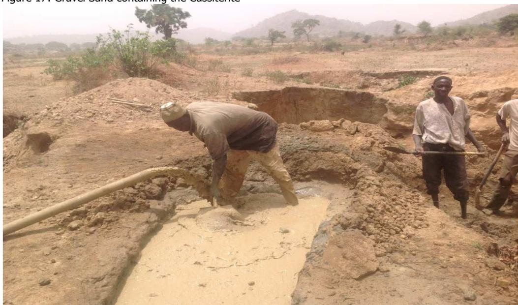
Figure 18: Local Separation of the Cassiterite from the gravel sand
