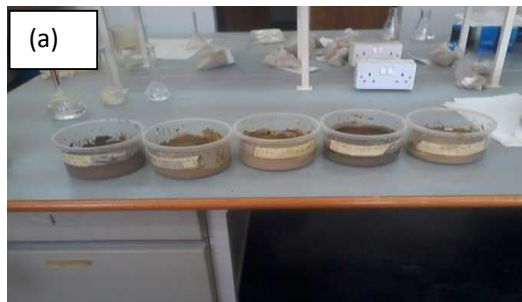
Plate I(a): Photograph of wet Bentonite undergoing CEC
