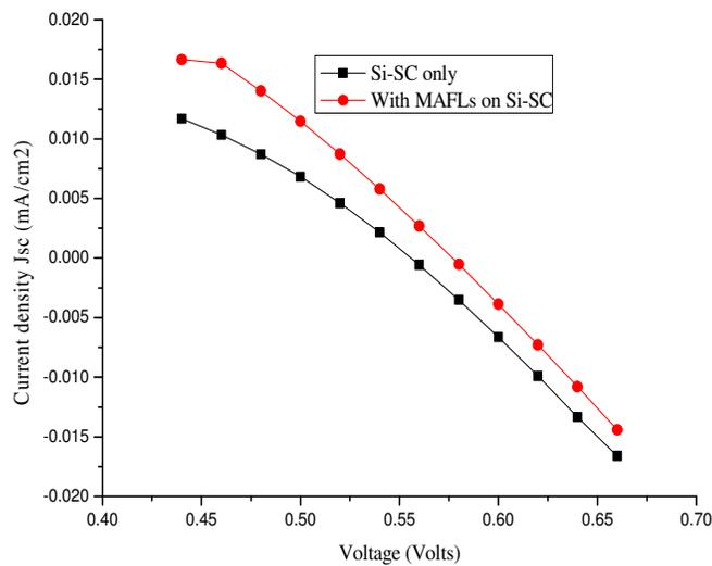
Figure 5: IV-characteristics of Si-Solar cells showing the effects of PMMA/SiO<sub>2</sub> Fresnel lenses array CPV-system in the improvement of the output characteristics of Si-Solar Cells.
