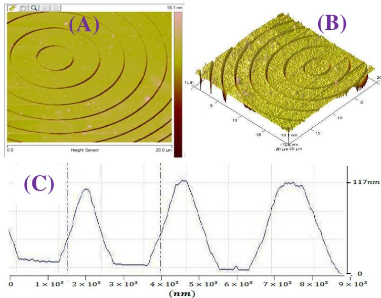
Figure 4: AFM images of surface topography and the etching profiles of Si-Fresnel rings (A) 2-D view (20  $\mu\text{m}$ )<sup>2</sup>(B)3-D view of the developed structures (20  $\mu\text{m}$ )<sup>2</sup>(C) Etching profiles.
