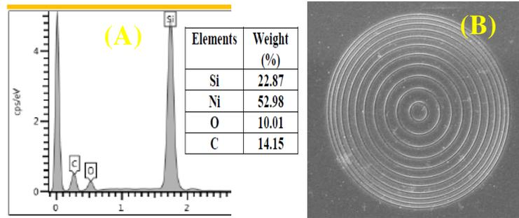
Figure3: FESEM images and EDX spectrum of the Fresnel rings on PMMA/Si surface (A) EDX spectrum showing the % weight of the elements detected (B) FESEM image of the Fresnel rings on PMMA/Si surface
