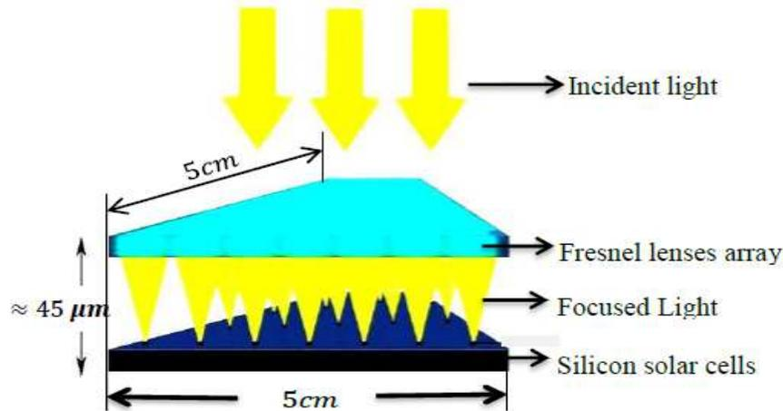
Figure 1: Schematic illustration of Micro array of PMMA/SiO<sub>2</sub> Fresnel lenses CPV-system on Si solar cells.
