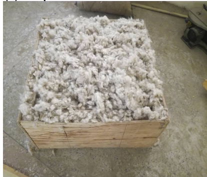
(c) Solar box filled Kapok insulator
