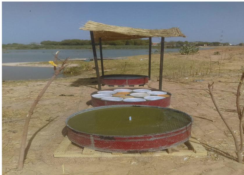
Figure 2. Experimental set up of the evaporation pans.
