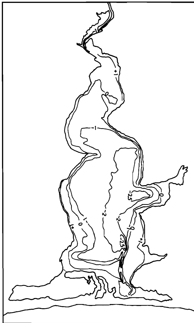
Figure 2 Bathymetric chart of the Bot River estuary (April 1980). Depth contours are in metres relative to mean sea level.
