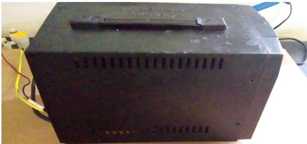
Figure 10 fully coupled 1KVA Solar Inverter
