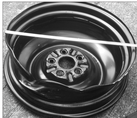
Figure 7: The black metal rim that impacted the victim. Note the depression on one side
