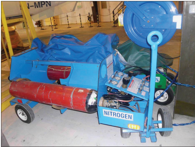
Figure 8: The high pressure nitrogen gas booster (TRONAIR) normally used to inflate aircraft tyres. Note the chain linking the equipment to the pillar on the right
