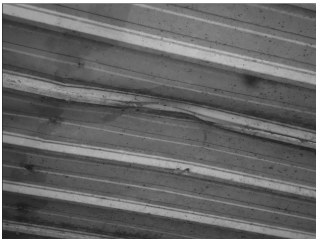
Figure 6: The incomplete circular impression on the aluminium ceiling; the arrow points at the dent caused by the impact
