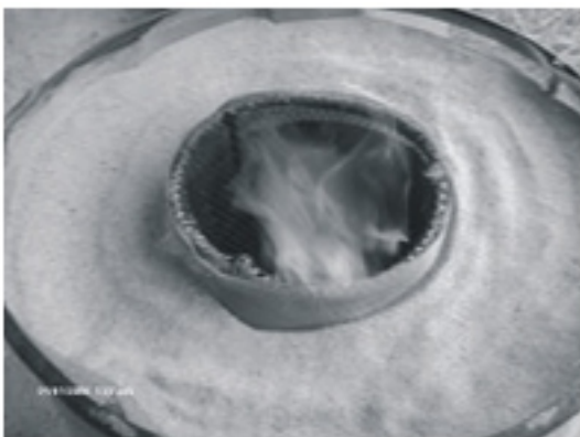
Figure 2. Inner steel mesh basket charged with red hot charcoal
