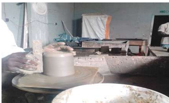
Plate I: A model of crucible being produced for slip casting
