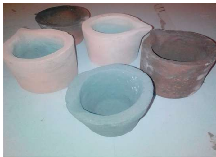
Plate III: Graphite crucibles before and after been fired
