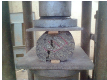
Plate 4: Strength test on papercrete specimen
