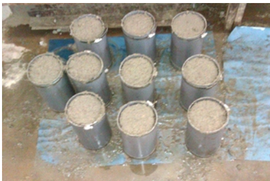
Plate 3: Pumice papercrete specimens
