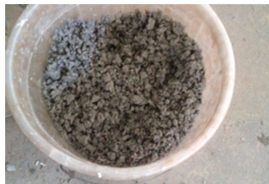
Plate 2: Water drained from ground newspaper
