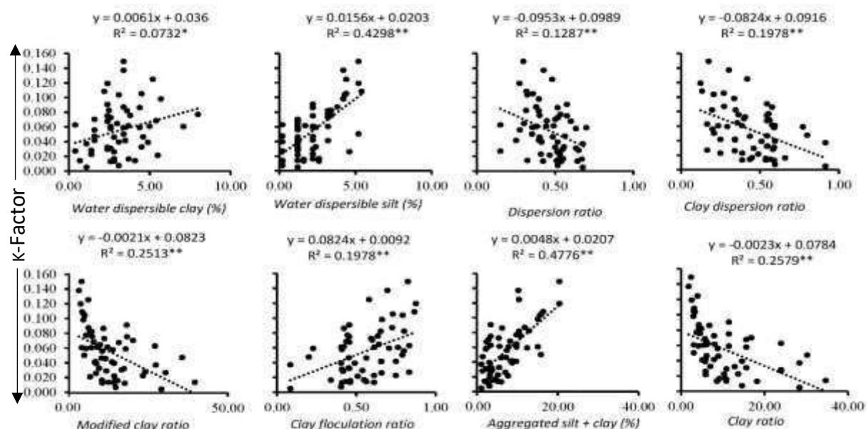
Figure 4: Linear regression of erodibility factor, K, on indices of microaggregate stability
