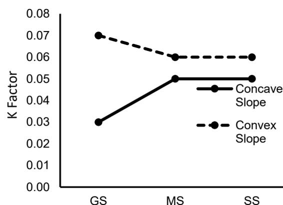
**Figure 2:** Interaction effect of slope curvature and gradient on erodibility factor, K
