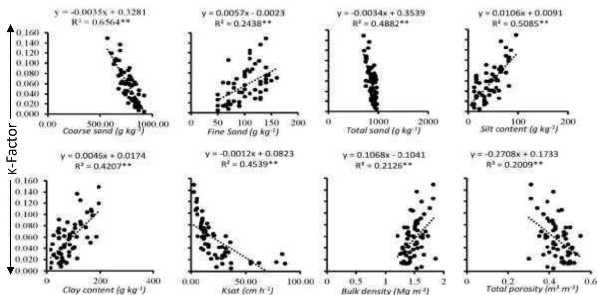
Figure 3: Linear regression of erodibility factor, K, on soil physical properties
