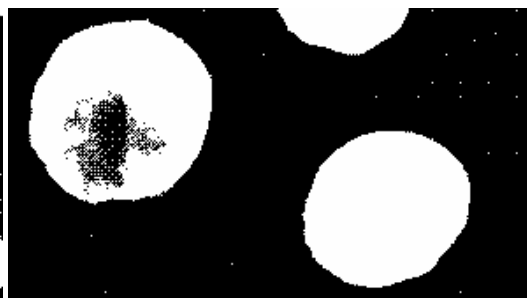
Figure 7: Scanning electron micrograph of stearic acid aerosols generated at 300 °C
