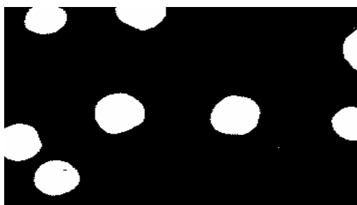
Figure 8: Scanning electron micrograph of stearic acid aerosols generated at 275 °C
