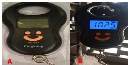
Figure 3: A - Digital weighing scale, and B - display of the animal's weight on the scale
