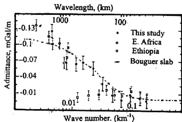
Figure 5. Comparison of admittance values of the Adamawa Dome (solid circle) and those of East Africa (open circles) and Ethiopian plateau (open rectangles) taken from Ebinger (1991). Errors bars are one standard deviation
