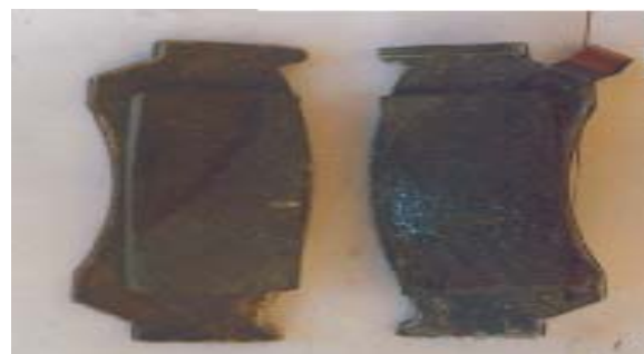
Figure 4. Worn samples of Kenaf Brake Pads fitted on back plates
