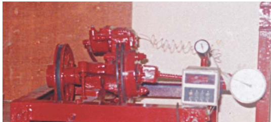
Figure 3. Experimental set up of the Friction Test Rig (FTR)
