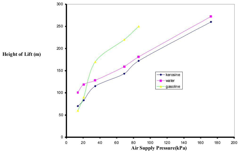
Figure 3: Plot of Lift against Supply Pressure for Different Fluids
