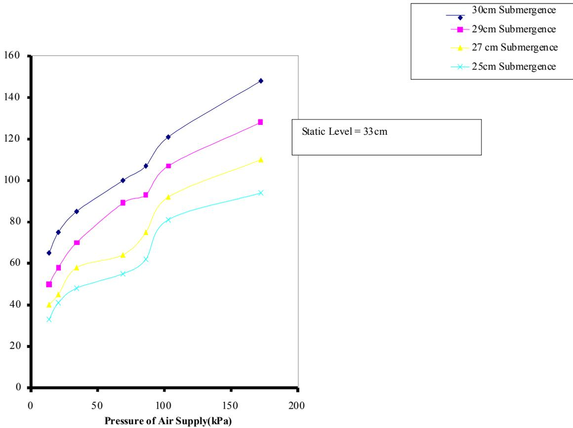
Figure 4: Plot of Water Lift against Air Supply Pressure in Sand-Water Medium
