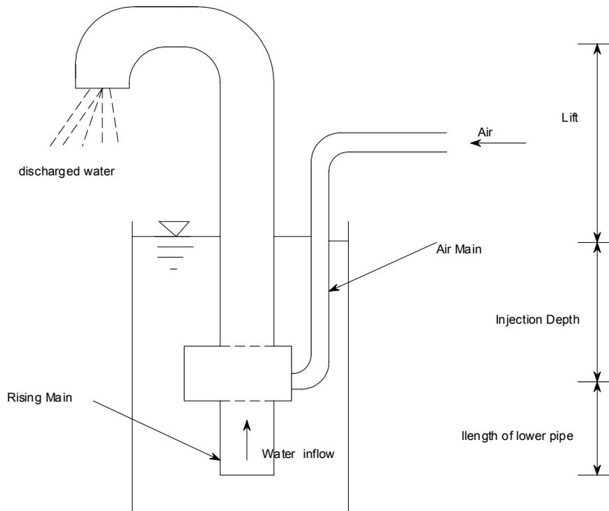
Figure 1: Schematic View of the Model Rig
