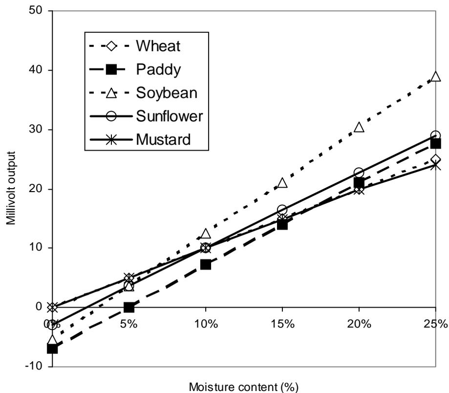
Figure 4: The moisture content calibration curves for different types of grains
