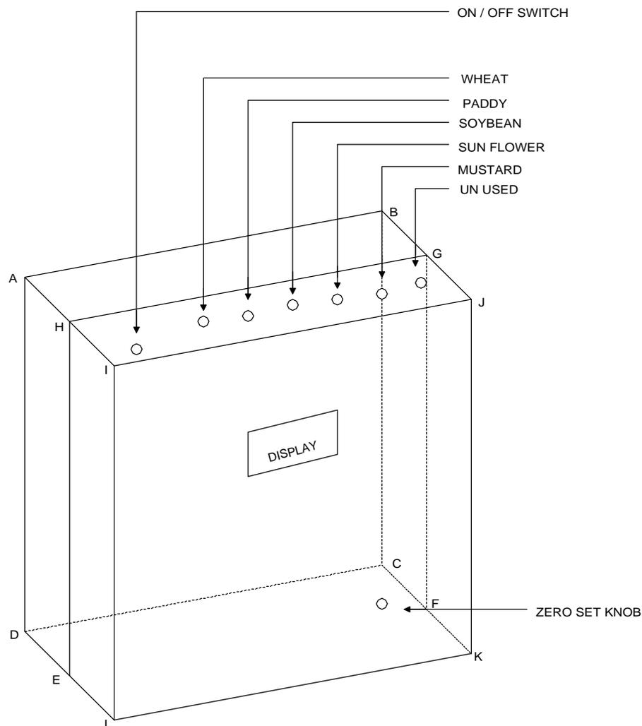
**Fig. 3: The schematic diagram of the grain moisture meter**
