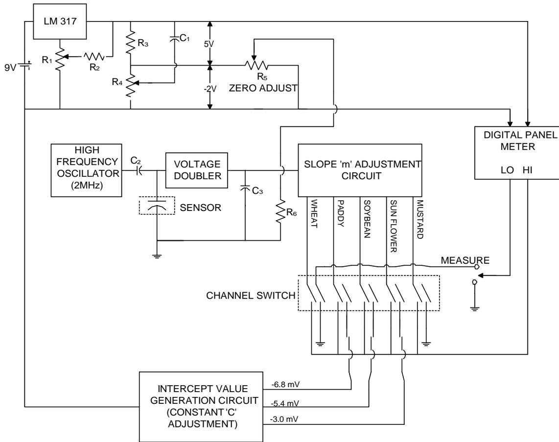
Figure 2: The electronic circuit of the grain moisture meter
