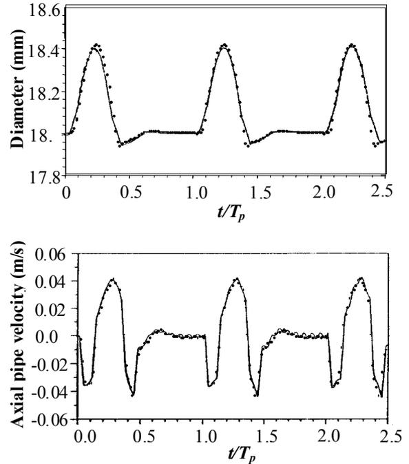
Figure 1: Predicted parameters at the mid point of the tube: — solution of Stuckenbruck, [7]; ... present solution based on finite elements formulation
