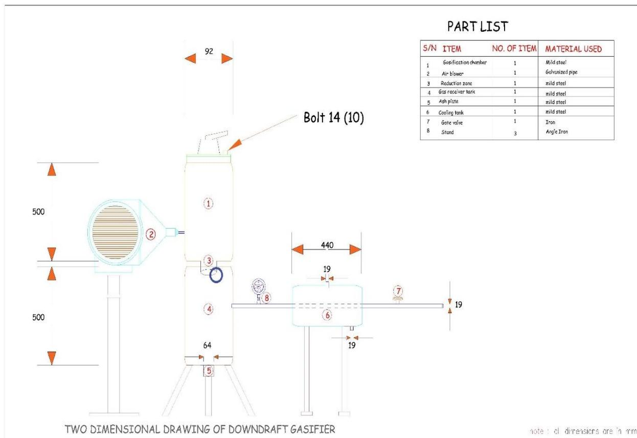
**Fig. 1: An orthographic working assembly drawing of the downdraft gasifier**
