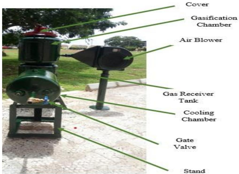
Plate 1: Assembled downdraft gasifier
