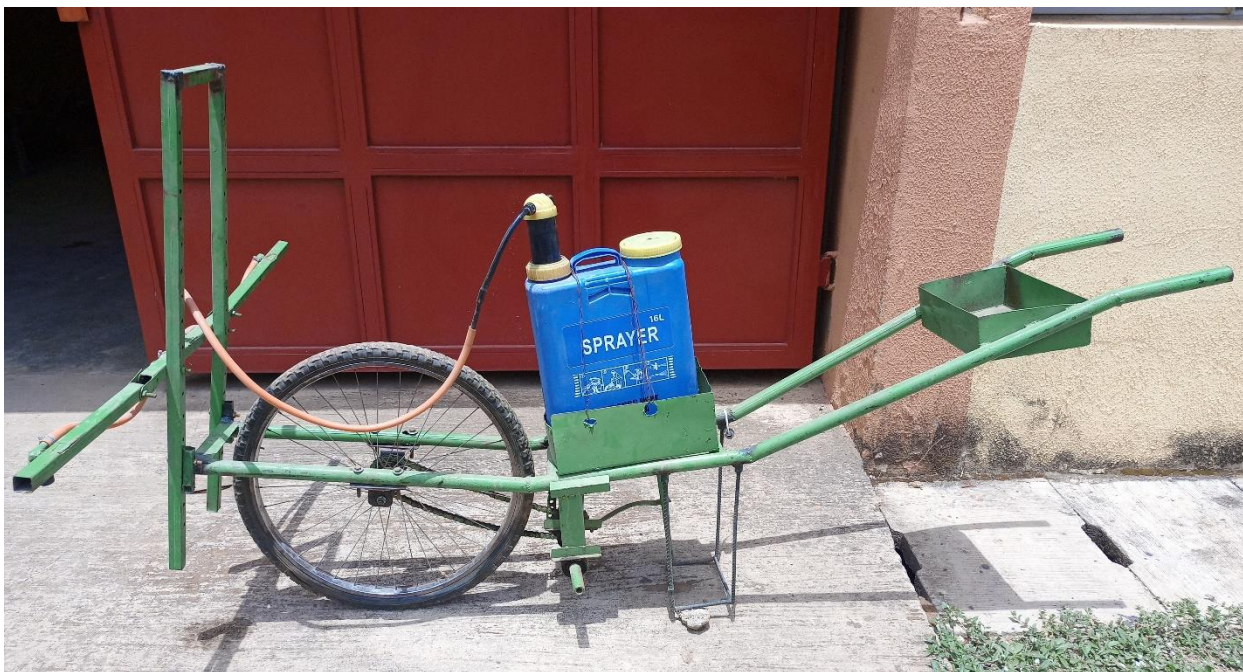
Plate 1: Pictorial representation of the developed hand-pushed pesticides sprayer
