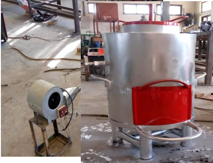
Plate 4: The produced crucible furnace before and after painting
