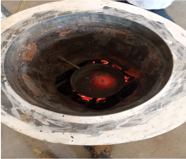
Plate 5: Melting of 5kg aluminum –scrap
