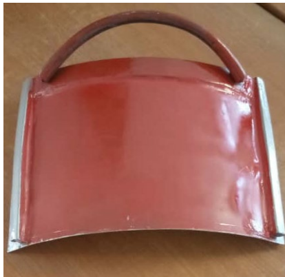
Plate 3e: Cover for the fuel port.
