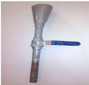
Plate 3c: Coupling from blower to burner.
