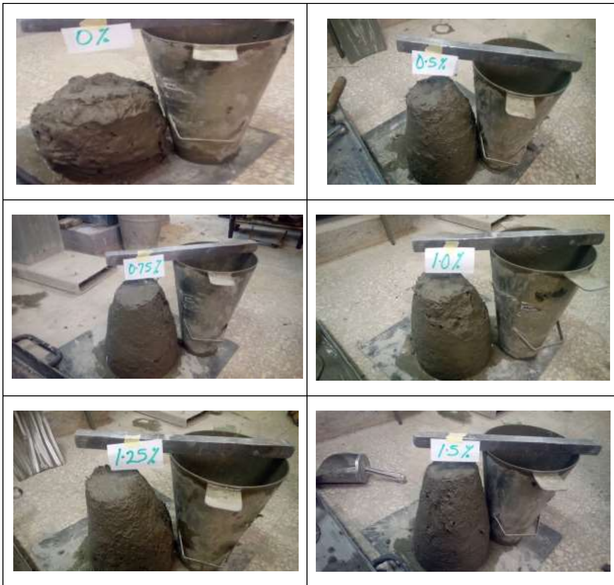
Fig. 5: Slump of Mixes with different Fibre Content
