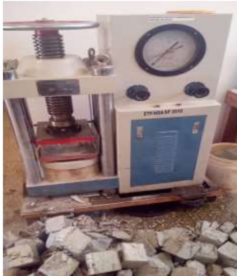
Fig 4: Compressive & Flexural Tensile Strength Tests Set Up
