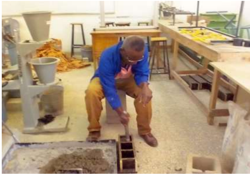
Fig. 3: Casting of Concrete Cubes for Compressive Strength
