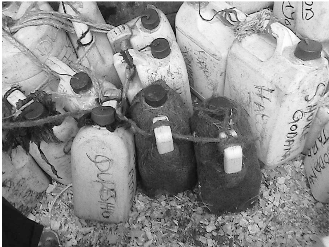
Figure 1: The 3 litre plastic milk containers, with and without moistened hemp. (Photo credit: AO Adongo Contact: adongoam@yahoo.co.uk )
