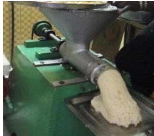
Figure 1 b: Mechanized system of fufu preparation
