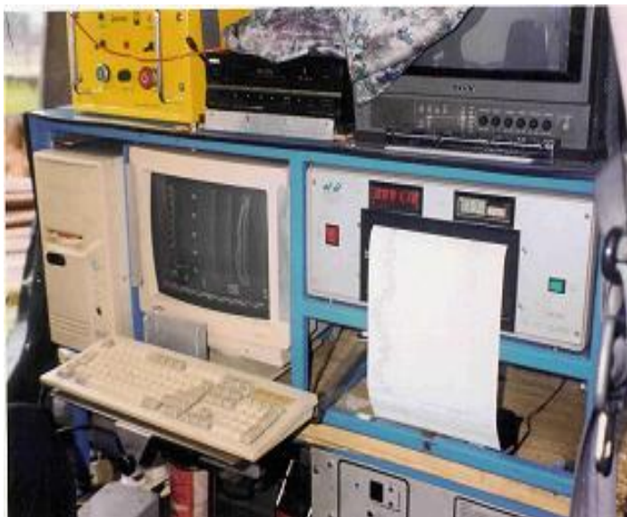
Plate 1. The RG PC Logger II™ Unit mounted on sports utility vehicle used for borehole loggings utilized for the study.
