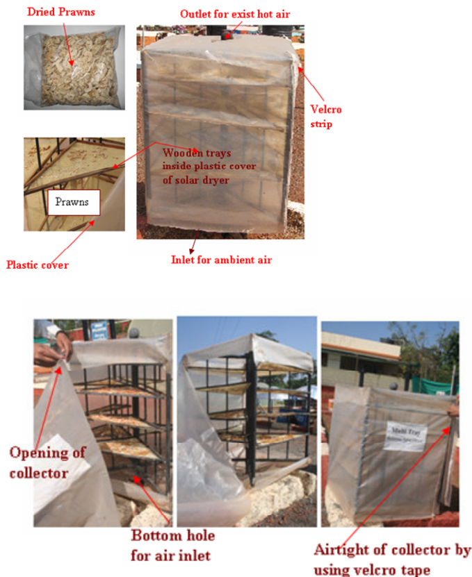
Figure 2. Vertical rotary low cost solar dryer.
