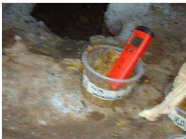
Figure 3. On-site measurement of FS pH.
