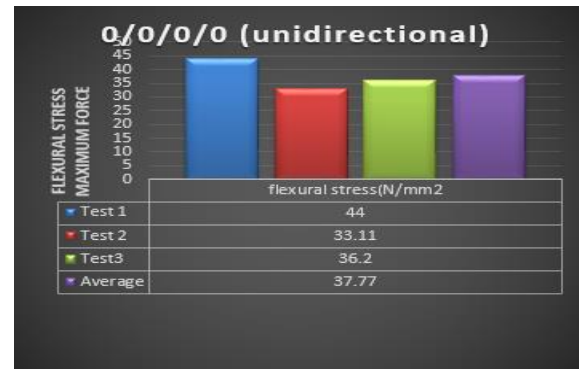
Fig 5. Flexural strength of the unidirectional system composites
