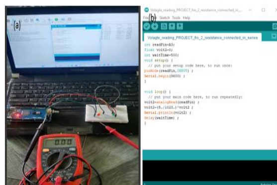
Fig. 5(a) Mechanism of Conductive fabric measurement Fig. 5(b) Voltage reading code via Arduino uno
