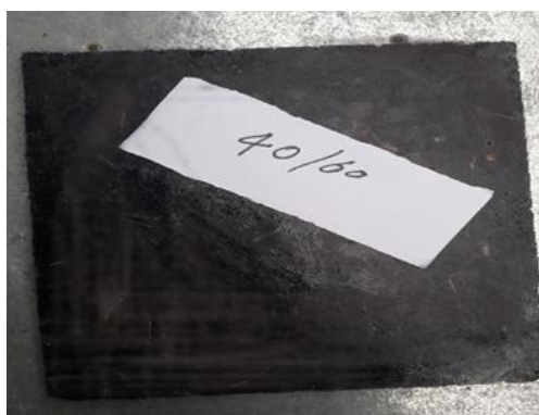
Fig 3b. Sample created with a composition of 40% human hair and 60% resin and filler
