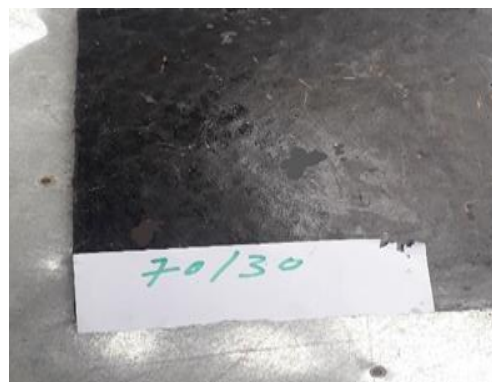
Fig 3d. Sample created with a composition of 70% human hair and 30% resin and filler
