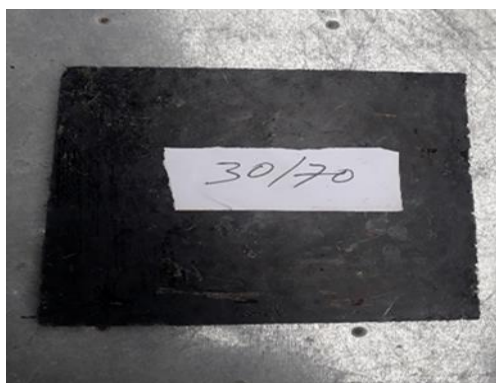
Fig 3a. Sample created with a composition of 30% human hair and 70% resin and filler.
