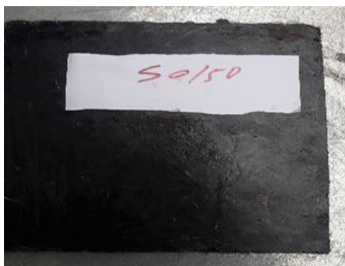
Fig 3c. Sample created with a composition of 50% human hair and 50% resin and filler.
