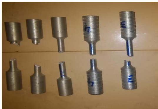
Fig.2: Tested tensile test samples
