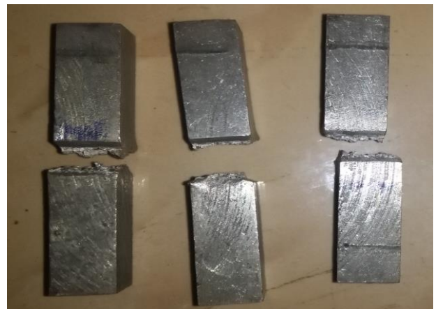
Fig.4: Tested impact test samples
