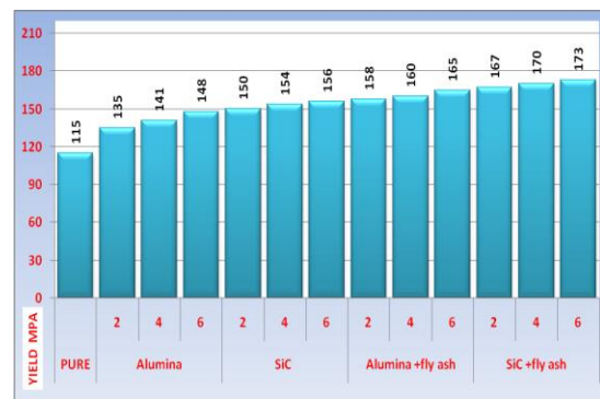
Fig.5: Yield strength of Al6065- SiC, Al6065- Al 2 O 3 , Al6065-Hybrid composites
