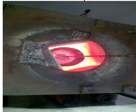
Fig.1: Stirring of the reinforcement
