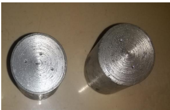
Fig.3 Tested hardness test sample
