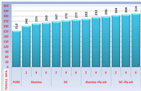
Fig.6: Tensile strength of Al6065- SiC, Al6065- Al 2 O 3 , Al6065-Hybrid composites
