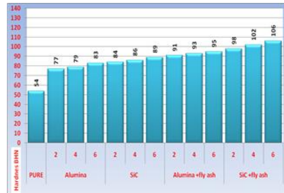
Fig.7: Hardness of Al6065- SiC, Al6065- Al 2 O 3 , Al6065-Hybrid composites
