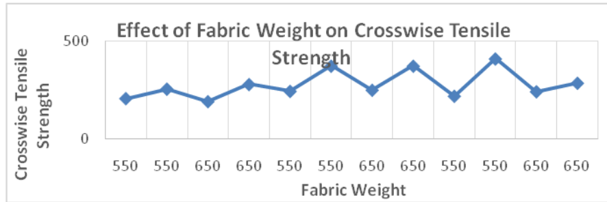
Fig. 5 Effect of Fabric Weight on Crosswise Tensile Strength
